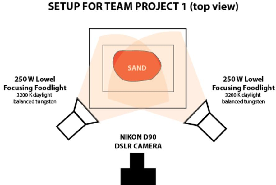
Figure 3: Diagram of setup.
